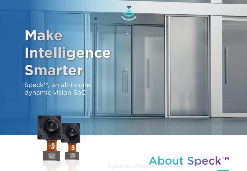
Speck<sup>™</sup> is a fully event-driven neuromorphic vision SoC. Speck<sup>™</sup> supports large-scale spiking convolutional neural networks (sCNNs) with a fully asynchronous chip computational architecture.
